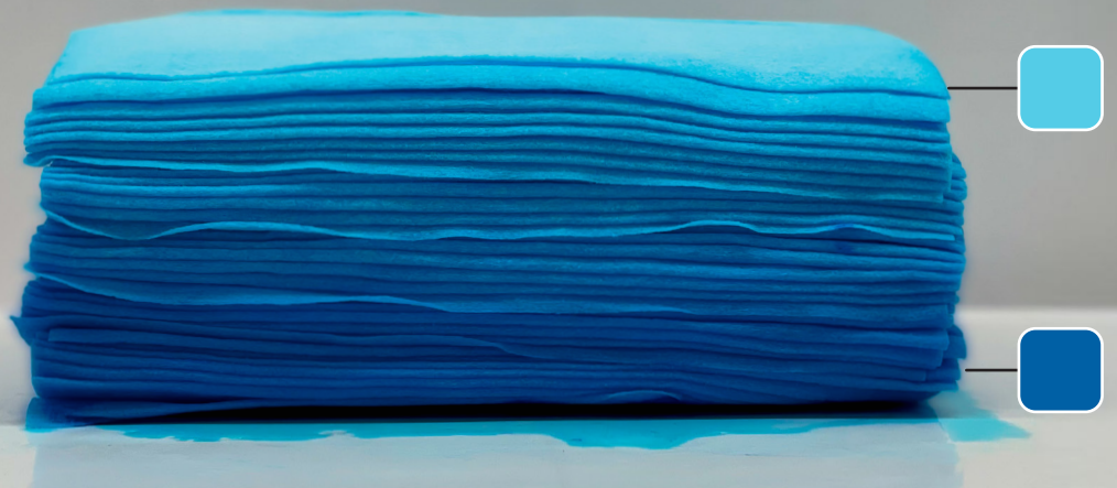
Figure 6: The disinfectant was coloured blue before impregnating a flowpack. After the flowpack had been stored for 3 days with the lid up, the stack of cloths was removed from the packaging and photographed.
