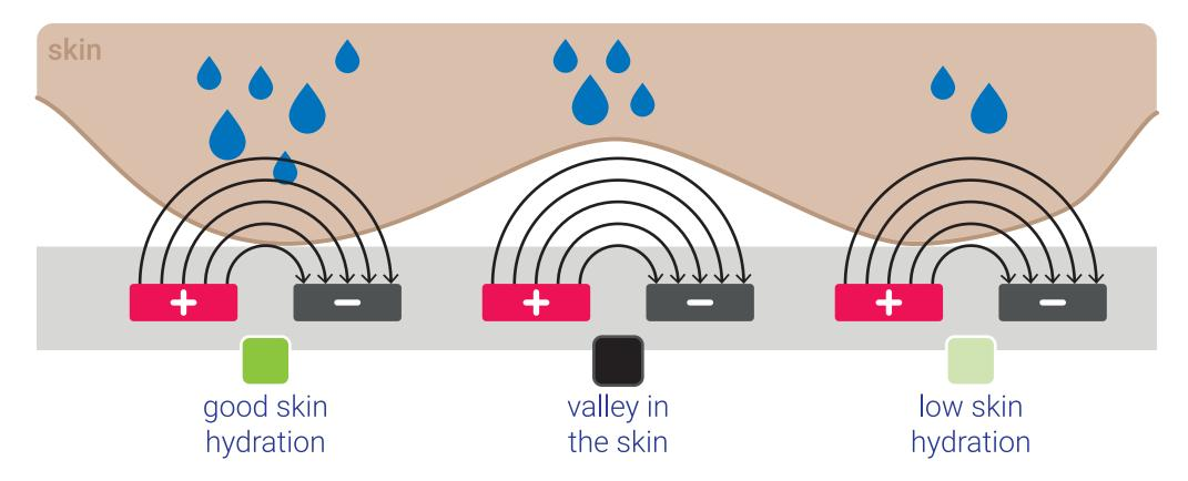
Capacitive Contact Imaging (CCI) is based on fingerprint sensor technology. 256×300 individual measurements (pixels) of the skin permittivity are recorded by generating electric fields, which are influenced by the water content of the top layer of the skin. The electric field values are then converted to skin hydration values and illustrative visualisations.
